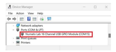
Once the port name is figured out, opening the port is very easy. The very first step is to load the Serial Port module and create an object that represents the serial port corresponding to the device. The following code does this. The exact value of the baud rate doesn't matter if it is a legal value. Also, use device names such as *COM15* on Windows and device node names such as */dev/ttyACM0* on Linux/Mac.
